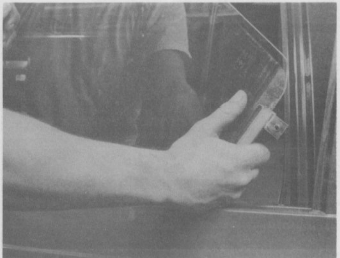
17.3b Remove the glass by carefully pulling it up – tilt it so it clears the channel
